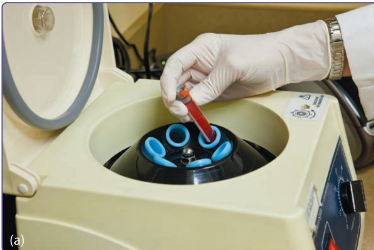
20-2 (a) Blood can be rapidly separated by spinning it in a centrifuge. (b) The erythrocytes (red blood cells) are at the bottom of the test tube.
